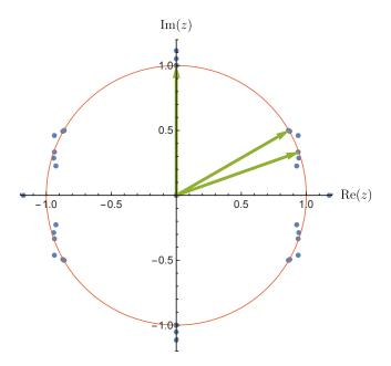
FIG. 15. Poles of the Padé-Borel approximation in the conformally mapped z plane. With N=50 terms, the first three Borel singularities can be resolved as accumulation points of Padé poles located on the unit circle at  $\theta=\pm\frac{\pi}{2},\pm\frac{\pi}{6},\pm\arctan\left(\frac{1}{2\sqrt{2}}\right)$ , denoted by the green arrows.
